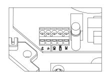
7. Test – place magnet next to reed, turn on, separate magnet from reed
